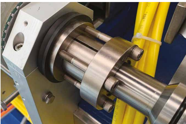
Locking two shafts using SIT-LOCK® 10, nickel-plated version.
