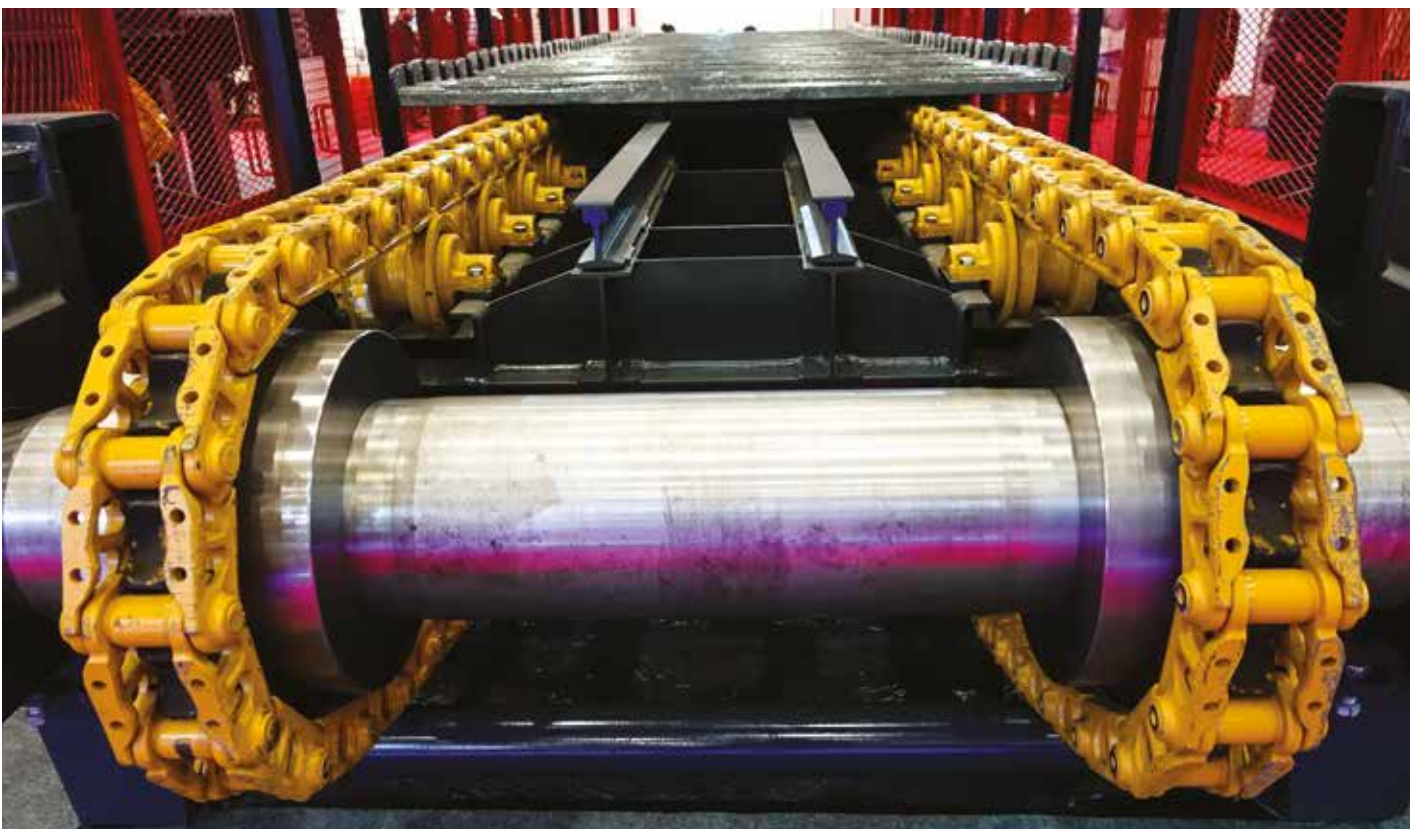
Locking conveyor chain wheels using SIT-LOCK® 4 COMPACT.
